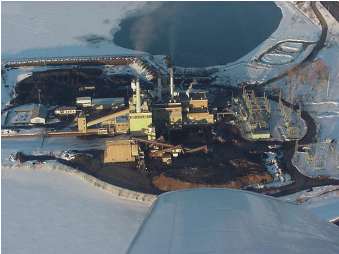
Figure 1. Aerial photo of the Bay Front Power Plant in Ashland, WI. The open water to the east of the plant is known as the hot pond and is the discharge point for the condensate cooling water.
