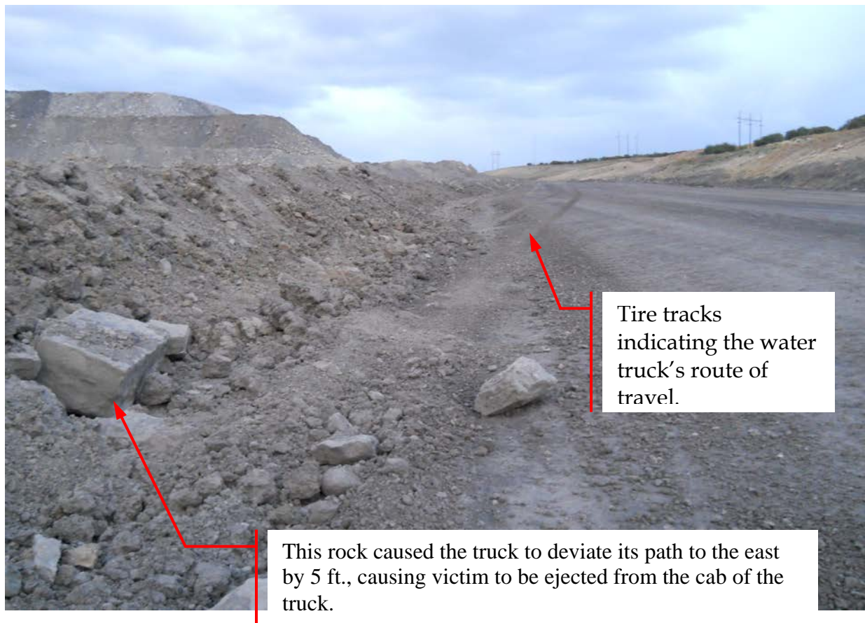
Figure 2: Site evidence of truck travel and cause of truck deviation.
