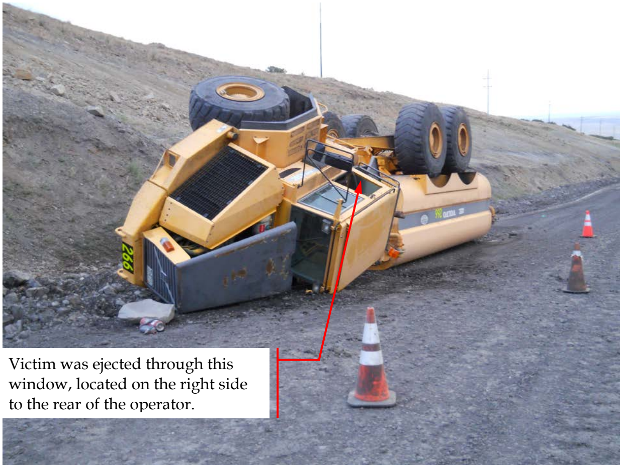
Figure 1: Overturned articulating water truck.
